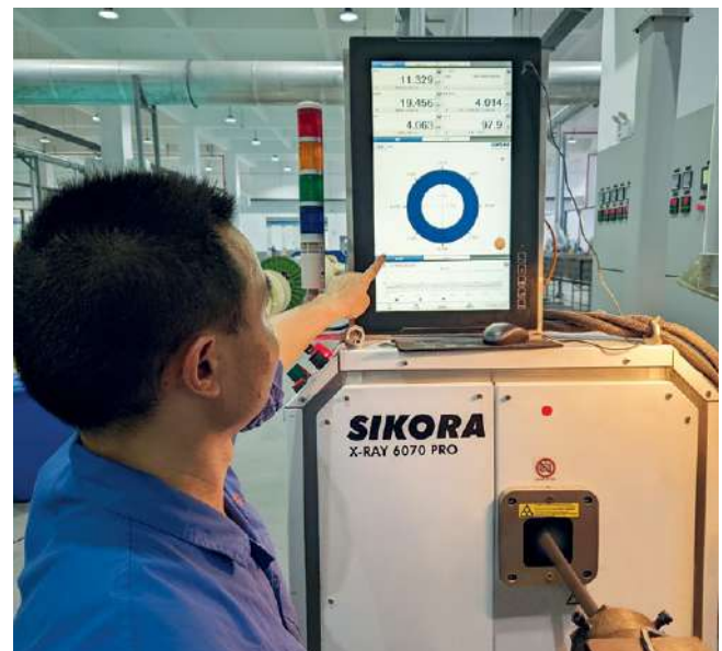
Wuxi Huacheng Cable uses SIKORA's X-RAY 6000 PRO for measuring and control during new energy cable production
