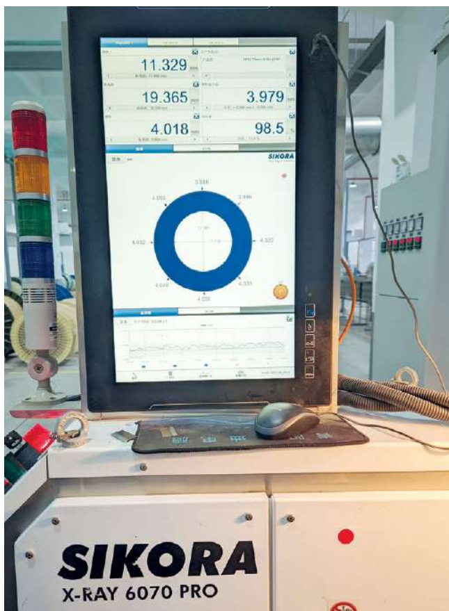
Wuxi Huacheng Cable uses SIKORA's X-RAY 6000 PRO for measuring and control during new energy cable production
