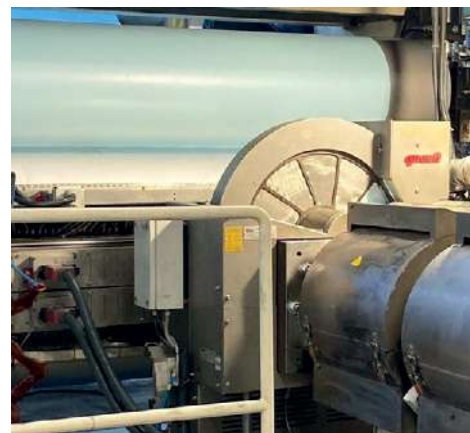
SFneos Filtration System in the production line of PVC film at Renolit
